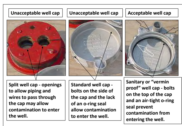
Figure 2: Photos of acceptable and unacceptable well caps
